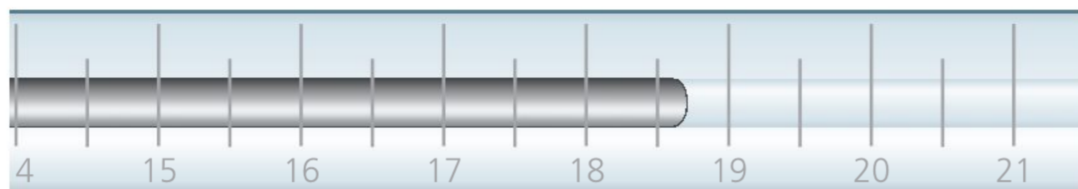
Figure 4.1 A magnified thermometer scale showing a temperature of 18.7°C: the last digit is uncertain
